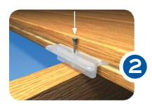
Step 2: Insert screws into Invisi-Fast Biscuit, place on joists in groove, do not tighten completely.
